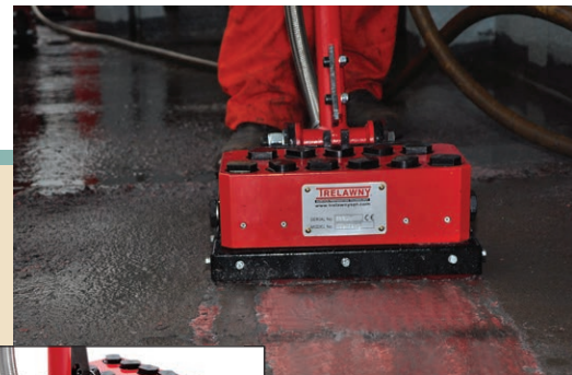
11 heads provide 33,000 BPM (11 x 3000 BPM)
