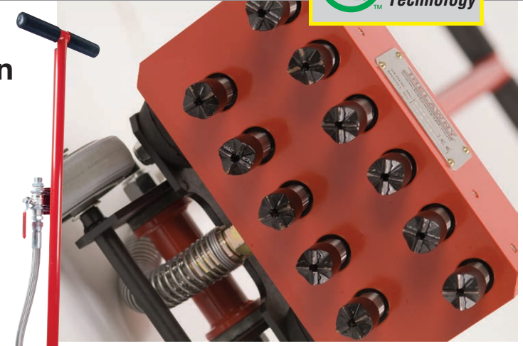
11 heads provide 33,000 BPM (11 x 3000 BPM)
