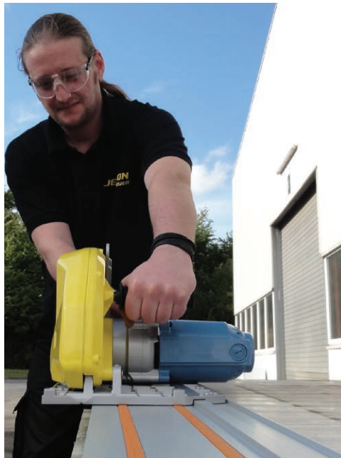
8320 SHDC Super Hand-Held Dry Cut Saw (608270 U) standard equipment includes a saw blade (P/N 608276).
